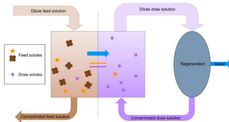
**Figure 2.** Forward Osmosis. Large volume of dilute wastewater (feed stream) enters. Lower volume of concentrated wastewater exits module. Water crosses the membrane due to osmotic pressure, diluting the draw solution. The draw solution can be regenerated by an external process, and the clean water stream removed. Some draw solute diffuses to the feed solution. Some feed stream components diffuse to the draw solution, where they may be concentrated by regeneration process.
