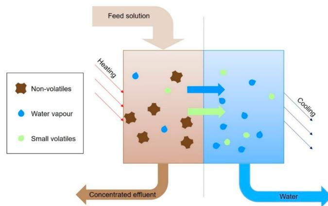
**Figure 3.** Membrane distillation. Large volume of dilute wastewater enters. A lower volume of concentrated wastewater exits the module, after addition of heat allows water vapour and other volatiles to cross the membrane. Heat is removed on the condenser side, and vapours condense into the water stream.
